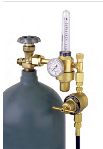
Fig. 2 — A typical flowmeter regulator is a fixed pressure/variable orifice device. Pressure is set at the factory to a compensated or calibrated pressure, depending on the flow range desired and the gases being used.
