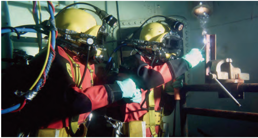
Fig. 5 — Two welder/divers in a practice tank for training and qualification. (Courtesy of the Royal Dutch Navy — Diving Group.)
