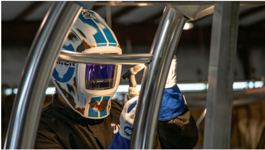
Fig. 1 — The GTAW process is often used in high-profile applications that prioritize weld aesthetics, quality, and integrity.
