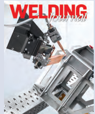
On the cover: TRUMPF's FusionLine enables users to add wire to their weld joint and bridge an opening up to 1 mm. (Source: TRUMPF Group.)
