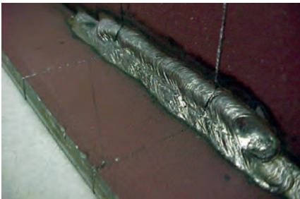
Fig. 7 — A three-pass fillet weld appearance after welding and cleaning. (Courtesy of the Royal Dutch Navy — Diving Group.)
