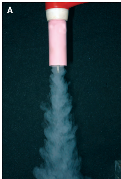
Fig. 4 — A gas lens increases shielding gas coverage and reduces turbulence compared to a collet body: A — Collet body in use; B — gas lens in use.
