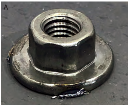
Fig. 5 — Overheated weld showing a large HAZ.
