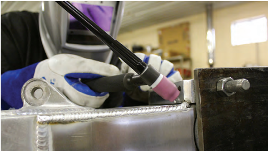
Fig. 2 — The GTAW process requires an inert atmosphere to protect the tungsten and the molten pool.
