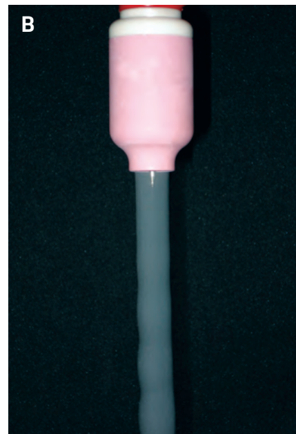
Fig. 4 — A gas lens increases shielding gas coverage and reduces turbulence compared to a collet body: A — Collet body in use; B — gas lens in use.
