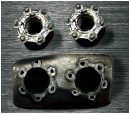
Fig. 5 — Overheated weld showing a large HAZ.
