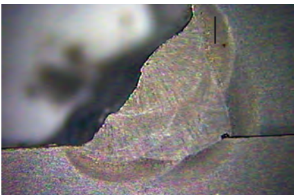
Fig. 8 — The cross section of the three-pass fillet weld, perfect profile, and penetration. (Courtesy of the Royal Dutch Navy — Diving Group.)
