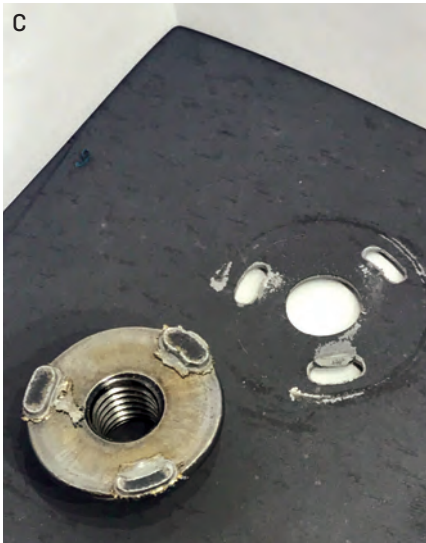
Fig. 6 — A — Showing almost no HAZ; B — showing bottom side again with almost no HAZ; C — showing nugget pull with almost no HAZ.
